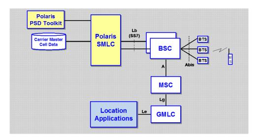
Figure 5. Reference Polaris WLS System Architecture for GSM
